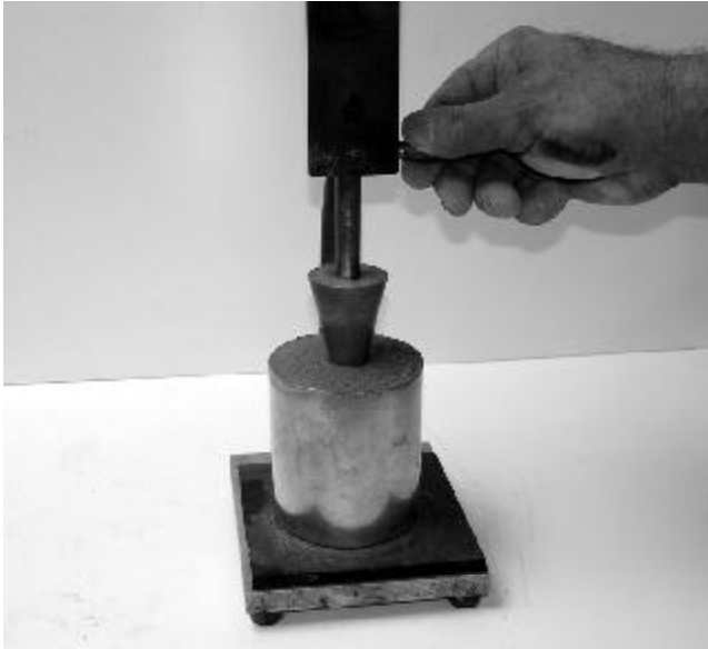
Figure 1—Mortar Consistency as Measured Using Cone Penetrometer
